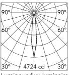
Luminous flux luminaire 419 lm
