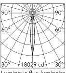
Luminous flux luminaire 1447 lm
