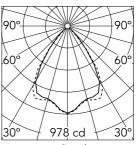
Luminous flux luminaire 1264 lm
