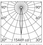
Luminous flux luminaire 1240 lm
