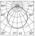
Luminous flux luminaire 855 lm
