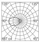
Luminous flux luminaire 580 lm
