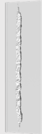
WALL RUPTURE WITH END CAPS
