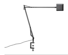
Adjustable table lamp providing direct light. Aluminium painted or chromed body, with die cast head, joints and forks, and extruded arms. Diffuser in photoengraved polycarbonate and aluminate on the perimeter. Edge Lighting technology light source. Optical switch sensor placed on the head that provide 3-step dimming function and color temperature adjustment at 2700K or 3200K. Power cord length 150 cm. Plug-in power supply with interchangeable plugs.
