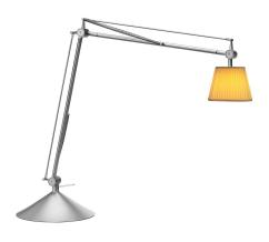
Task lamp providing direct and diffused light. Acid-etched pressed borosilicate glass internal diffuser. Plissé cloth external diffuser. Gray painted die-cast aluminum diffuser support. Gray painted assembly composed of extruded aluminum arms, steel tie rods, stainless steel springs, and 50% fiberglass reinforced, injection-molded polyamide joints. Gray painted die-cast Zamak BASE.
