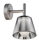
Wall sconce providing diffused lighting. Injection-molded polycarbonate external diffuser completely finished with highvacuum aluminization process. Gray painted die-cast aluminum diffuser and lamp support. Gray painted, injection-molded polycarbonate wall fitting and rose.
